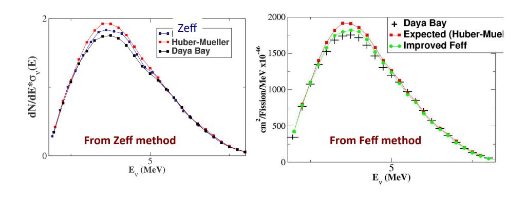
Both the magnitude and the shape of the predicted spectrum depends on the method used to obtain the average value of Z as a function of end-point energy - Improved descriptions tend to lower the expected antineutrnio spectrum
