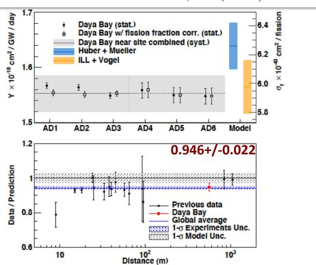
The very accurate measurement of the total flux at Daya Bay and RENO confirms the shortfall
