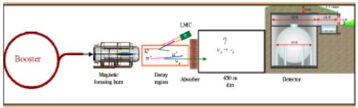
**Used the Booster Neutrino Beam at Fermilab**
