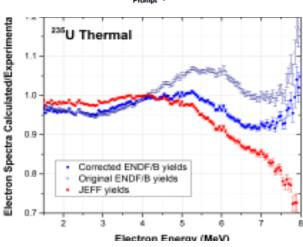
Dwyer and Langford pointed out that the ENDF database predicts an analogous bump in the beta-spectrum relative to Schreckenbach.
