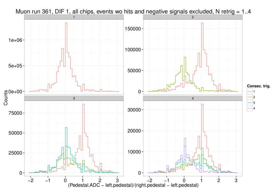
Fraction of right pedestals (ie. the ones which are closer to the right than to the left)
