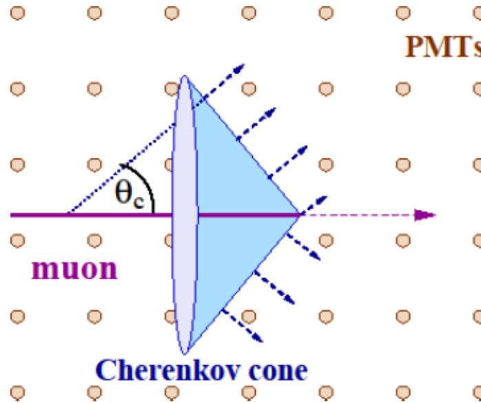
**PMTs** Muon track from CC muon neutrinos
