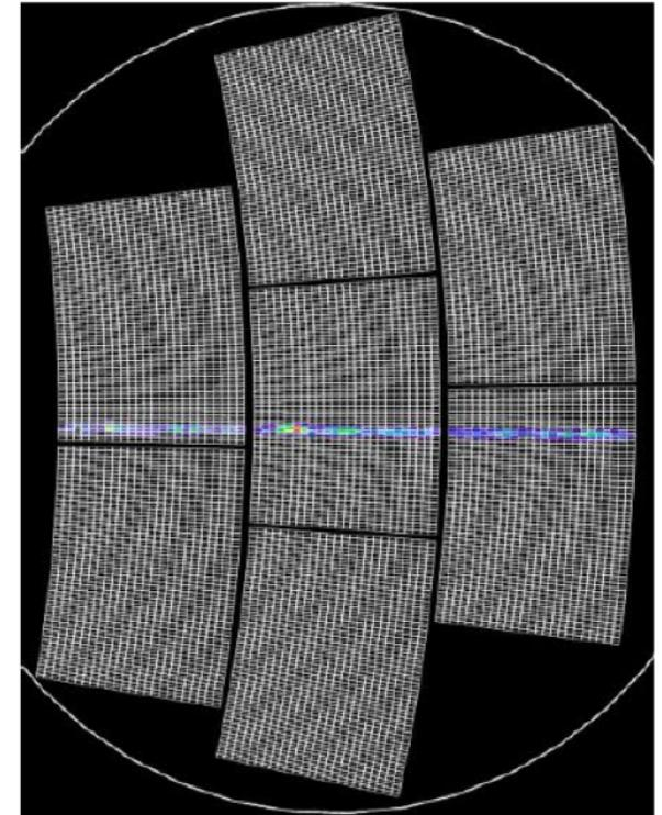
*A multi-module detector sensitive to misalignment and distortions*
