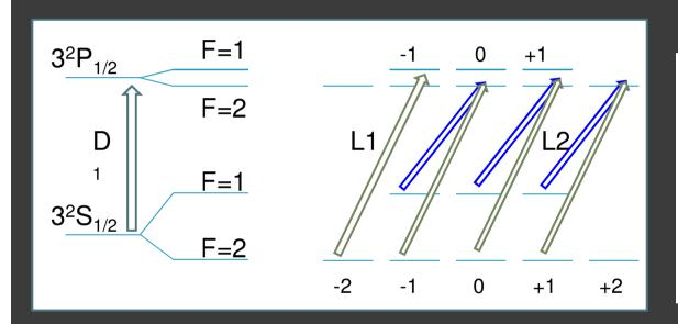
L1+L2 lasers using an optical modulator
