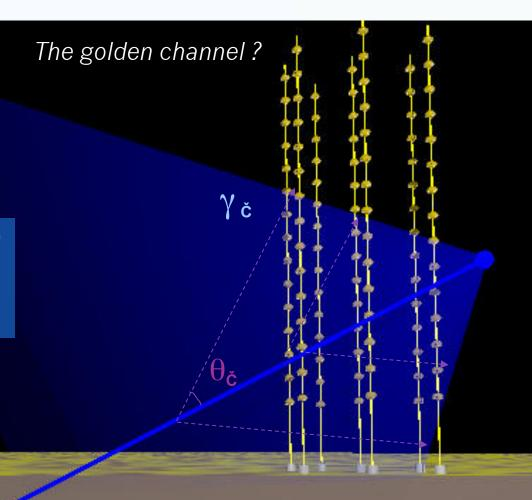
Time, position, amplitude of PMT pulses  $\Rightarrow \mu$  trajectory ( $\sim v < 0.5$ °)
