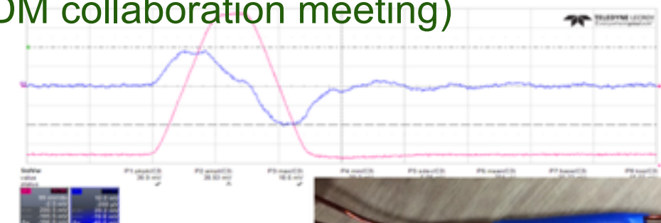
B-field measurement with pickup loop
