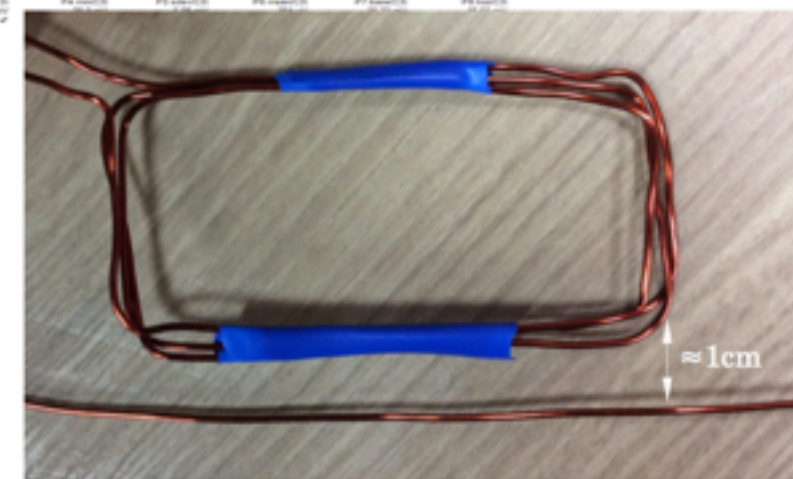
Current passes through the wire and the B-field is picked up by the loop
