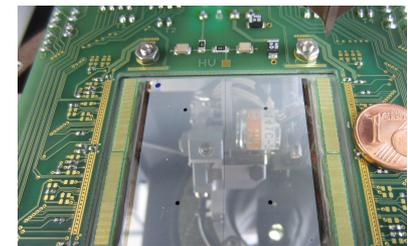
Hamamatsu KEK/Tsukuba : production of sensor wafer and 4chip card
