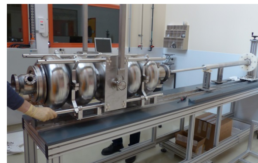
Cathode's insertion in horizontal position
