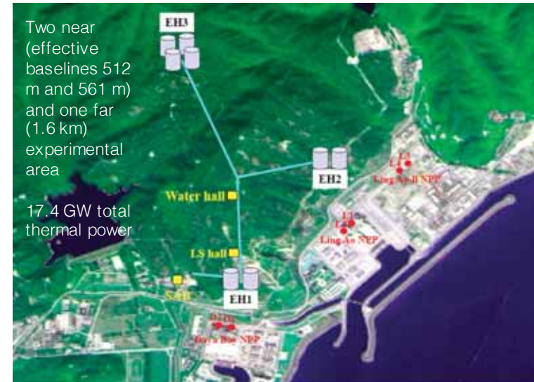
Layout of China-based Daya Bay experiment
