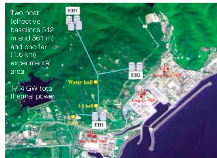
Layout of China-based Daya Bay experiment
