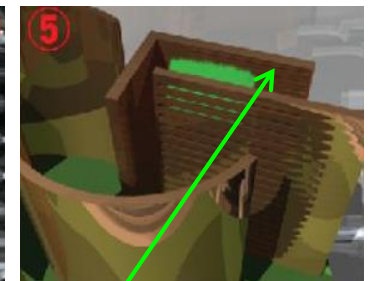
multiplication by n dynodes and signal on the anode
