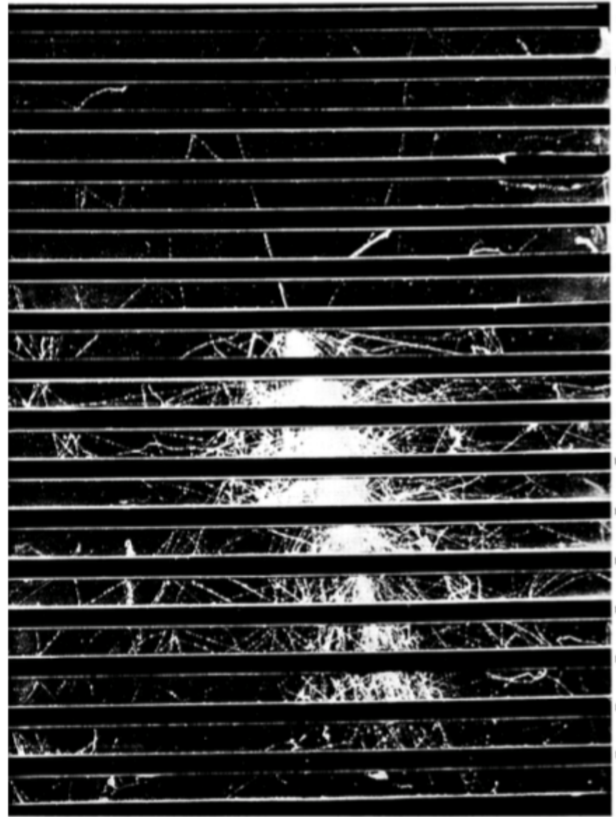
Fig. 1. Image of a particle cascade, or shower, as seen in a cloud chamber at 3027 m altitude. The primary particle is estimated to be a proton of about 10 GeV. The first interaction will most probably have been in one of the lead plates. Neutral pions feed the cascade which multiplies in the lead. Charged pions make similar interactions to protons, or decay into muons. The cross-sectional area of the cloud chamber is 0.5 \times 0.3 \text{ m}^2 and the lead absorbers have a thickness of 13 mm each [Fretter, 1949].
