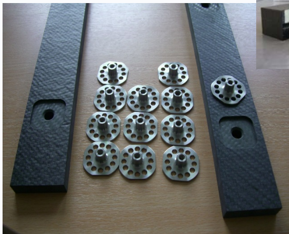
Dummy composite structures for plies' thickness validation
