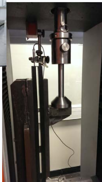
Shearing tests to determine stress in the structure
