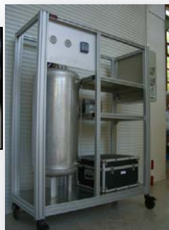
Cooling station Leakless loop
