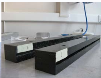
Dummy composite structures for plies' thickness validation
