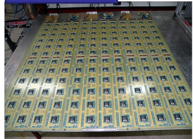
1m 2 equipped with 144 MICROROC
