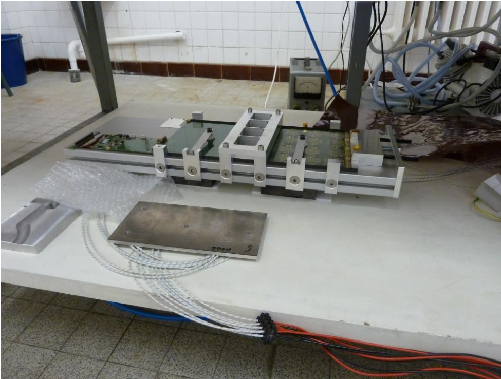
Layer remains in cradle during polymerisation
