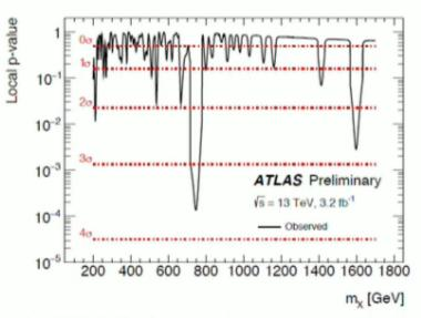
In the NWA fit the resolution uncertainty is profiled in the NWA fit and is pulled by  $1.2\sigma$
