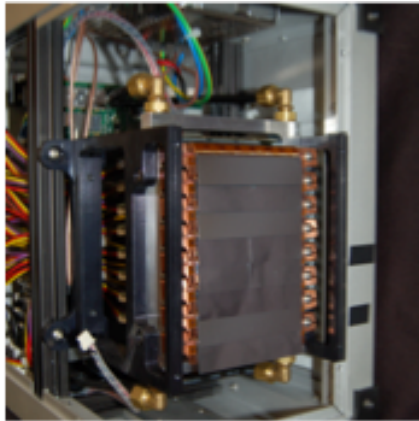
XPAD3 : 130 x 130 \mu\text{m}^2 pixels
