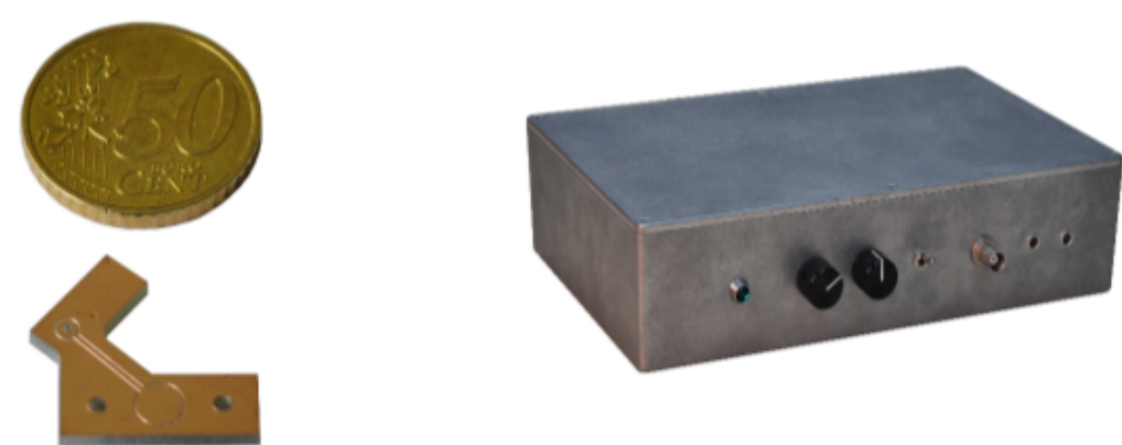
Sensitve element and dedicated electronic developed at LAPP for the sensors
