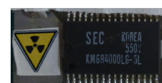
Old SRAM technology already tested at other 14MeV-neutron generators comparable to GENEPI2 (CEA Valduc, Sodern, Frascati)
