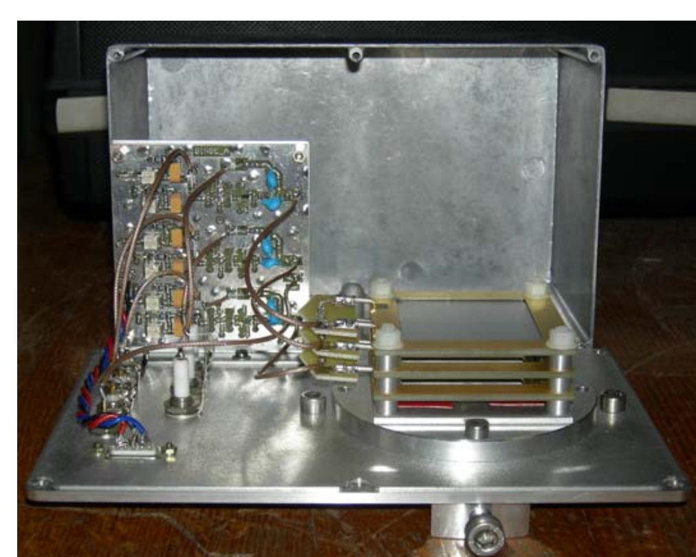
Schematics and picture of the proton telescope: a thin layer of CH2 allows the conversion of neutrons into protons (1 p for 10^3 incident n), then the energetic protons (en. > 9 MeV) are detected by a triple coincidence of the signals from 3 Si detectors (300, 500 and 1000μm).
