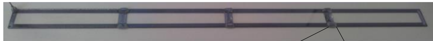
First prototype of microcooling stave 270 mm long.
