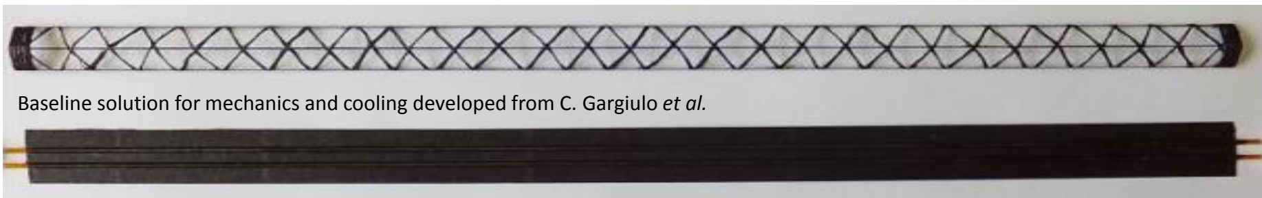
First prototype of microcooling stave 270 mm long.
