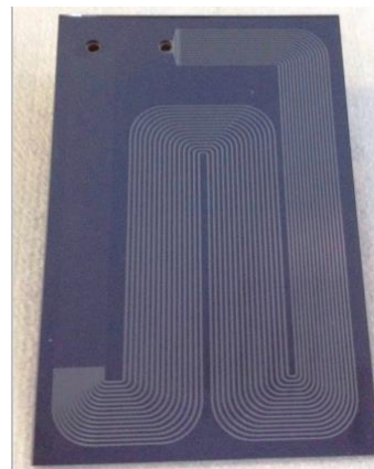
40x60 mm 2 Pyrex-silicon sample with simpler micro-channels pattern
