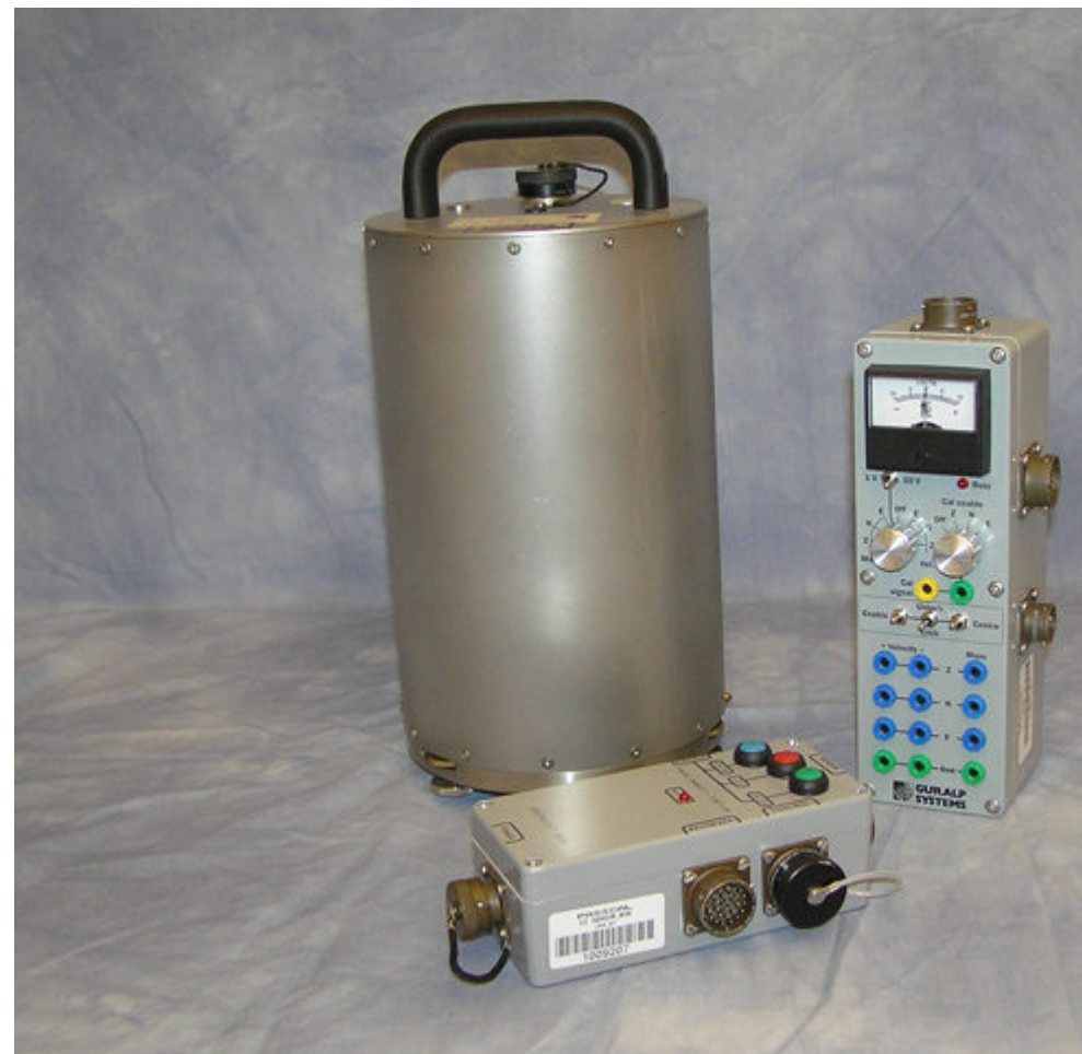
Guralp CMG-3T Broadband Sensor 120s - 50 Hz flat velocity response
