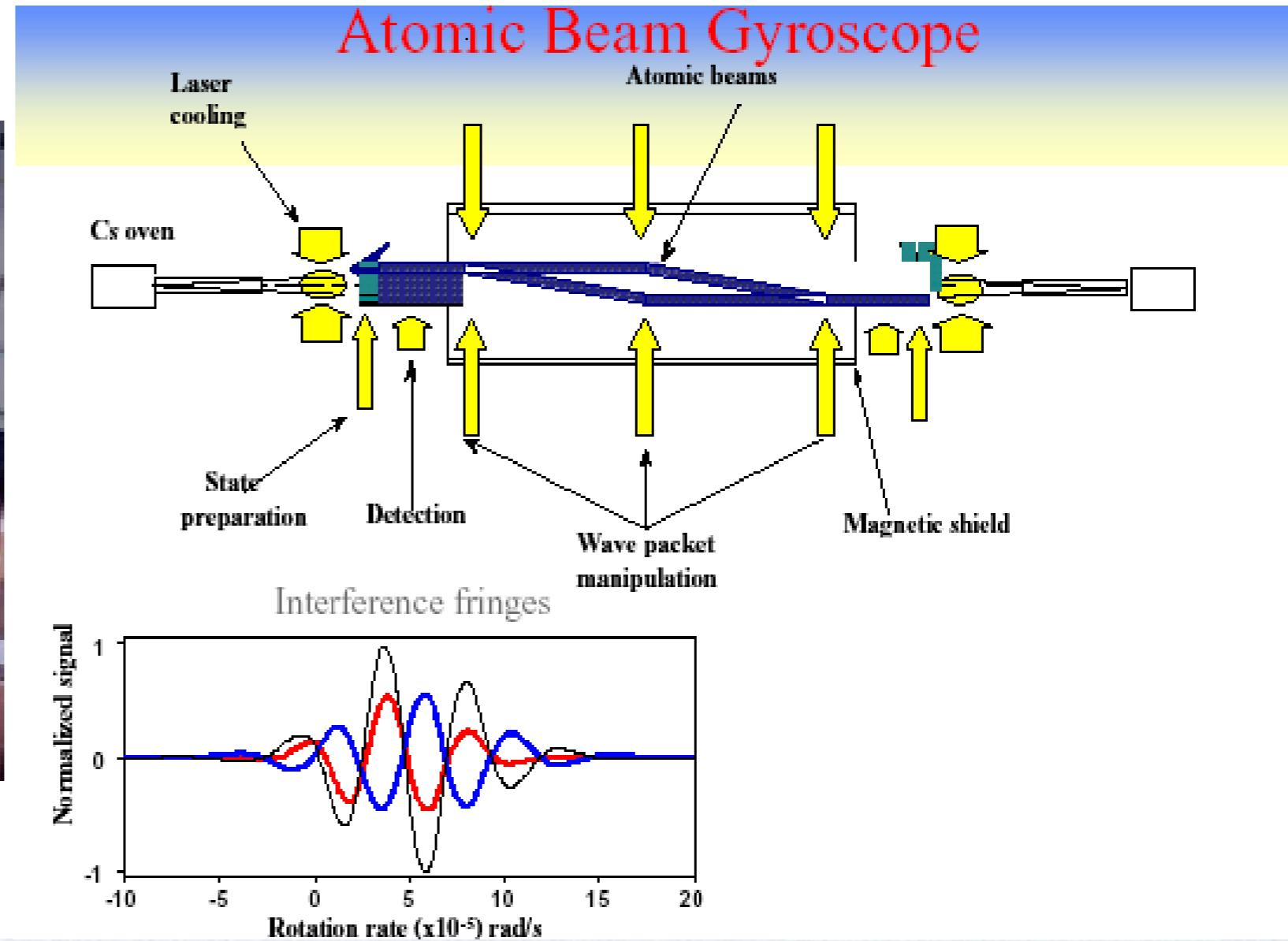
sensitivity:  $6 \times 10^{-10} \text{ rad} \cdot \text{s}^{-1} \sqrt{\text{Hz}}$
