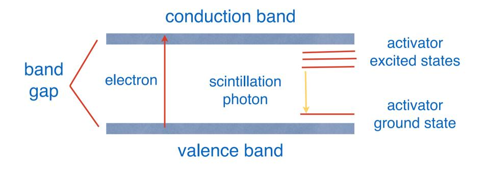
Nal (TI): 20 eV to create e<sup>-</sup>-hole pair, scintillation efficiency ~ 12%
