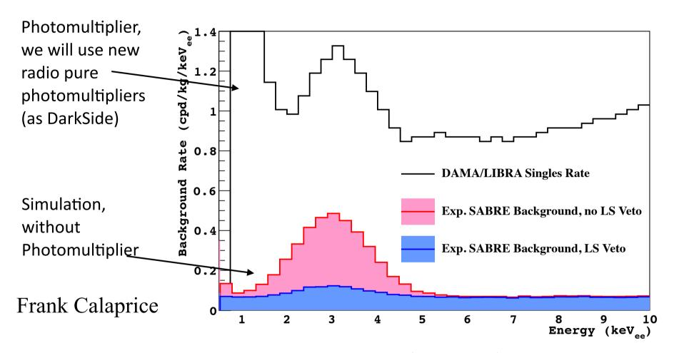
Assume the K level is the same as the powder (~10 ppb K); U (<1 ppt), Th (<1ppt), Rb (0.2 ppb) levels are measurements in recent crystal tests. External background is estimated to be relatively small compared to internal.
