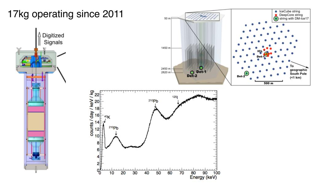
6.5-8.0 keVee region is measured to be  $7.9\pm0.4$  counts/day/keV/kg." Dominated by assembly housing and PMT - no ice contribution
