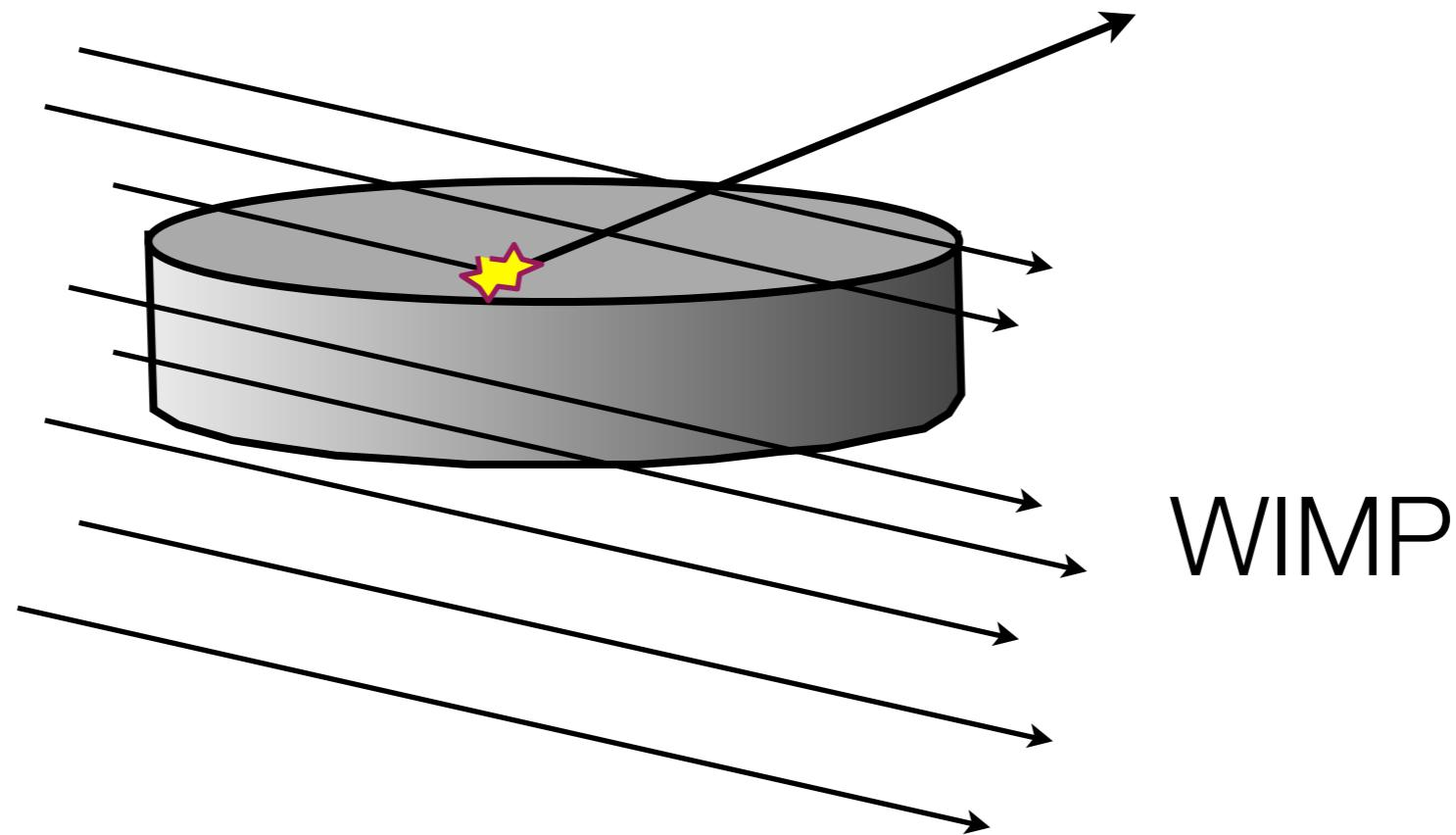
Cryogenic semiconductor detectors looking for
