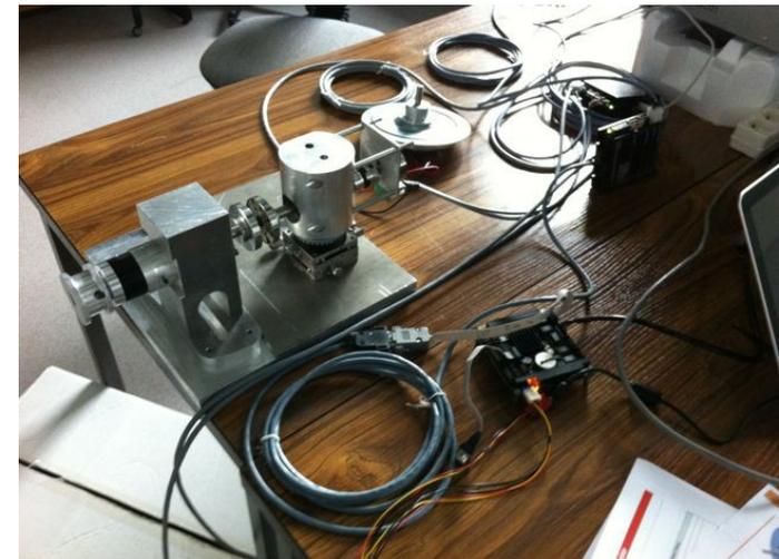
Spring 2012 : Control of the motor / magnetic transmission of the carousel-filter un-clamp system
