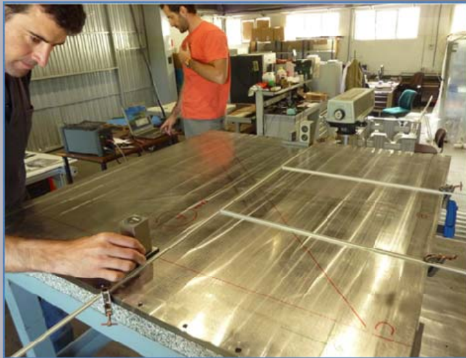
(Left-top) Measurement of a plate planarity using a laser interferometer system.
