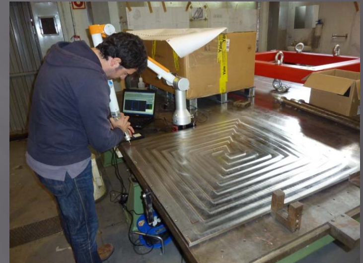
(Left-Bottom) Measurement of the m 3 prototype using the CMM arm on the assembly table.
