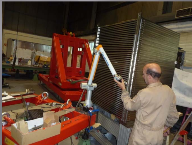
(Righth-top) Measurement of the plate using a CMM arm.
