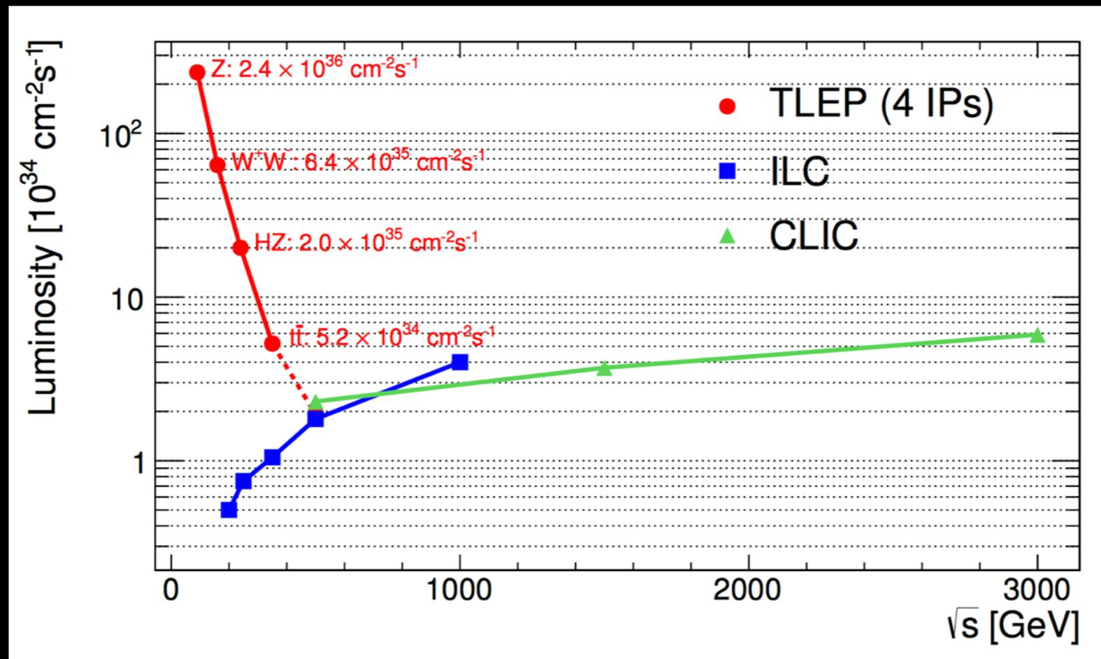
Instantaneous luminosity expected at FCC-ee, in a configuration with four interaction points operating simultaneously, as a function of the centre-of-mass energy.
