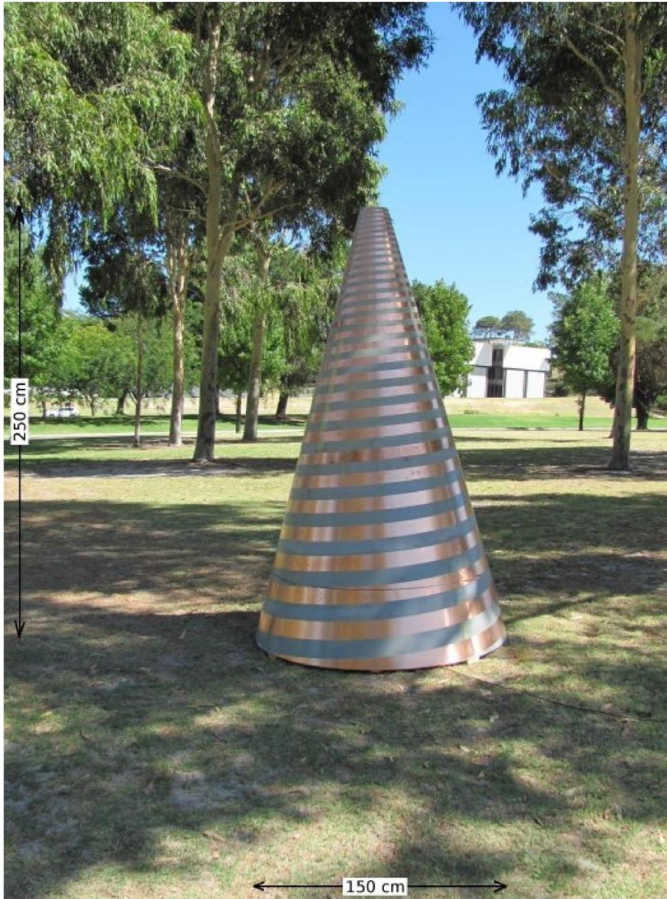
The broadband conical log spiral antenna
