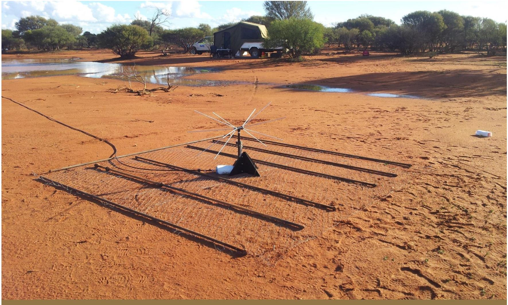
The broadband off-the-shell biconical antenna
