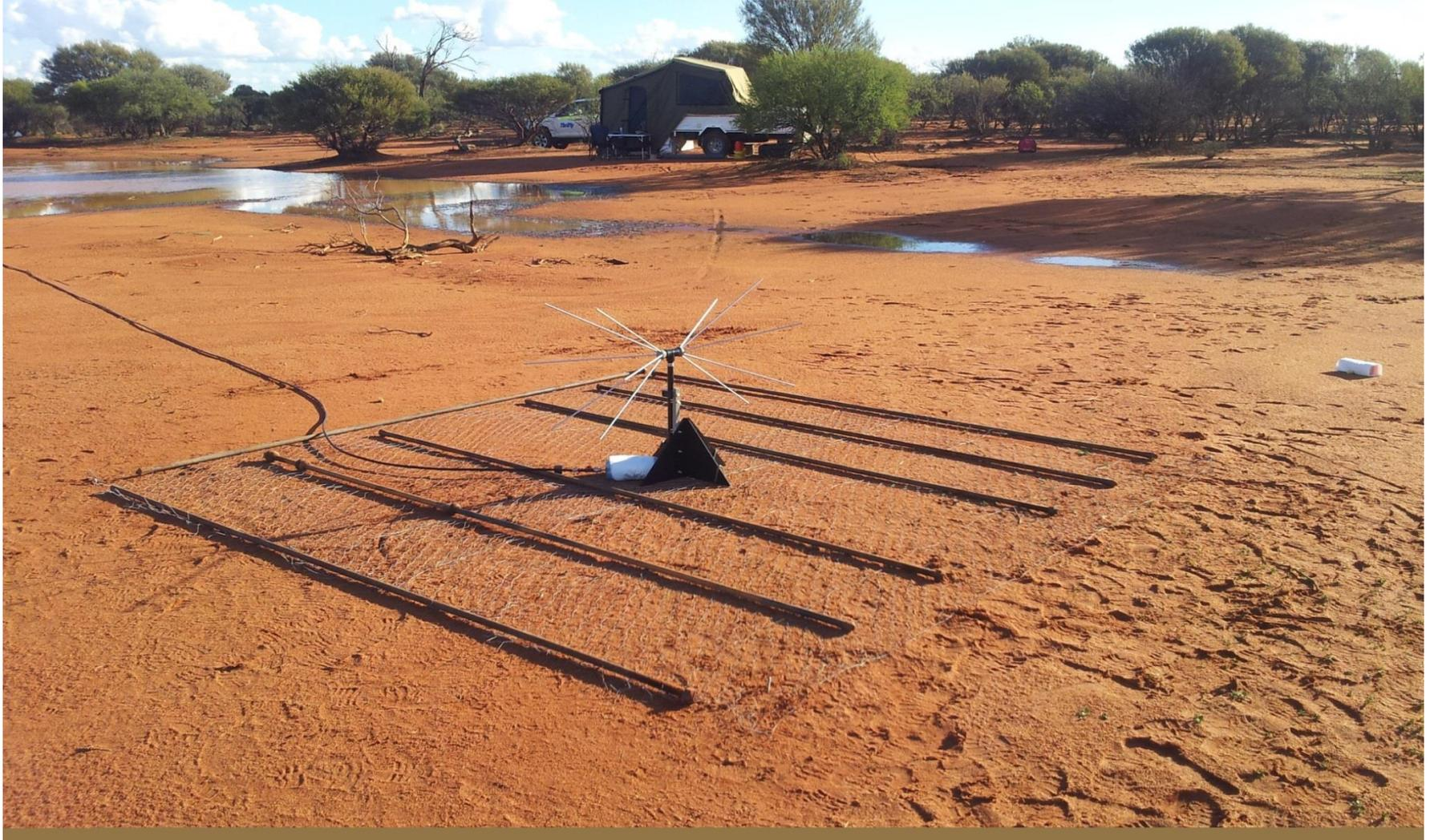
The broadband off-the-shell biconical antenna
