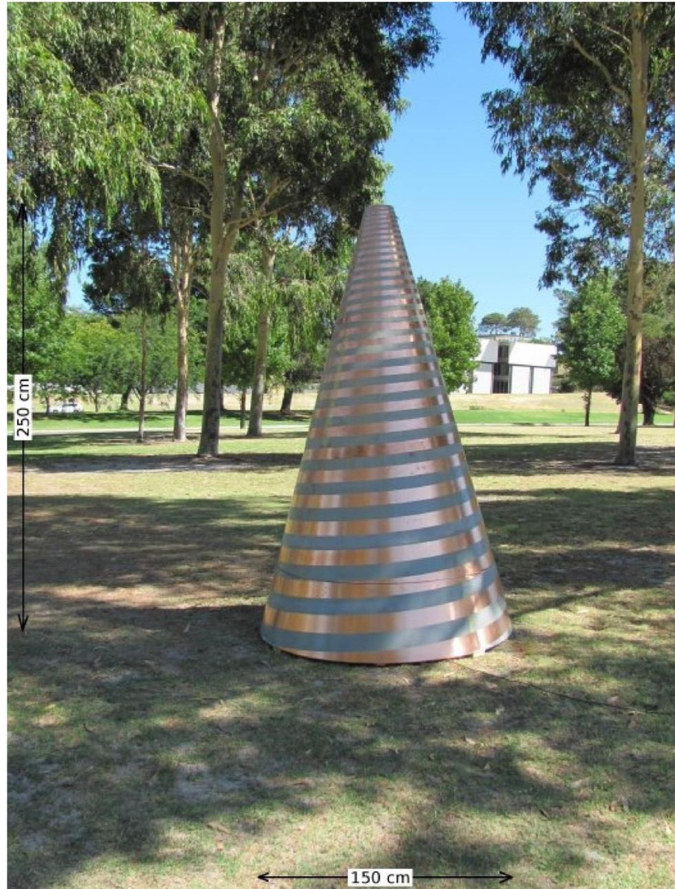
The broadband conical log spiral antenna
