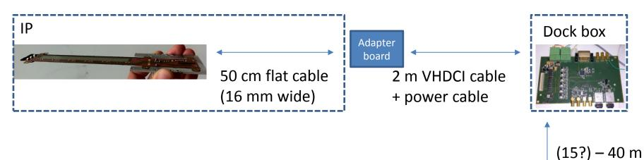
Our layout tries to imitate the VXD readout path to simplify system integration
