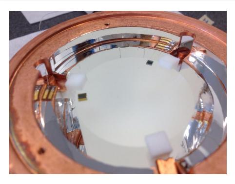
The cylindrical crystal with a size of  $\bigcirc 40 \times 40$  mm and a mass of approximately  $\sim 150$  g, was used in a scintillating bolometer.
