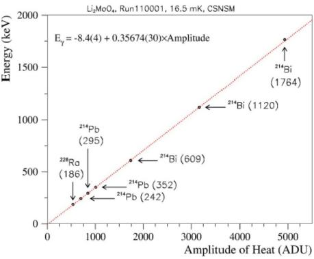
The calibration was made using the environmental radioactivity. The most dominant signals come from the Rn chain
