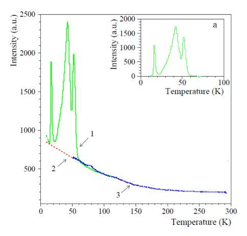
We have subtracted the thermo-stimulated luminescence (TLS) contribution assuming a linear dependence of the luminescence on temperature.
