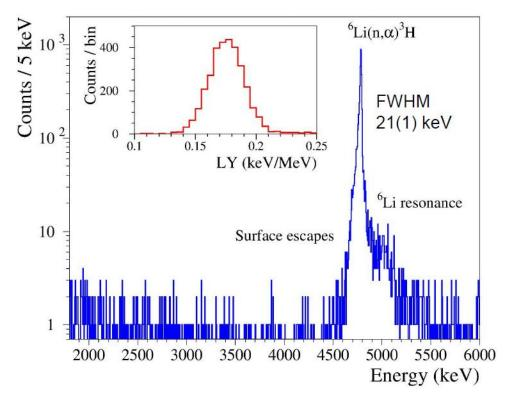
The light yield at the  $\alpha$ -triton peak (LY 0.17 keV/MeV) is significantly lower than that of fast electrons. The corresponding quenching factor of the mixed -triton events with respect to events is about 23% at  $\sim 4.8$  MeV.
