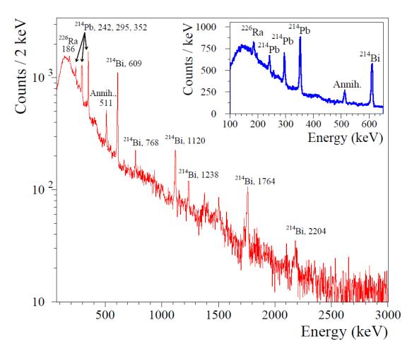
Energy spectrum measured in the Orsay aboveground set-up over 118 hours.
