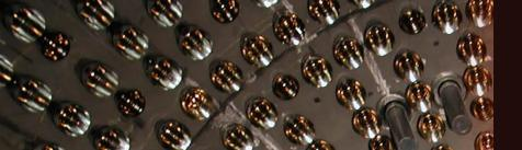
1<sup>st</sup> shield: 1000 tons of ultra-pure buffer liquid (pure PC) contained in a stainless steel sphere of 7 m radius;
