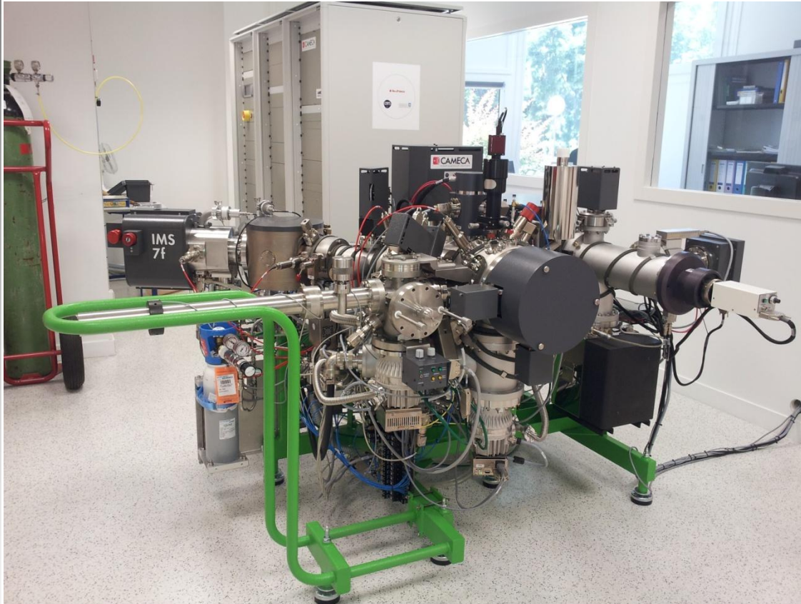
SIMS at GEMaC laboratory, Versailles Cameca IMS 7f
