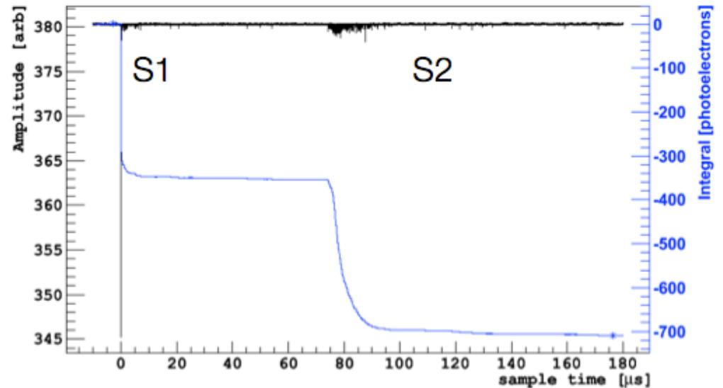
The time between the S1 and S2 signals gives the vertical position
