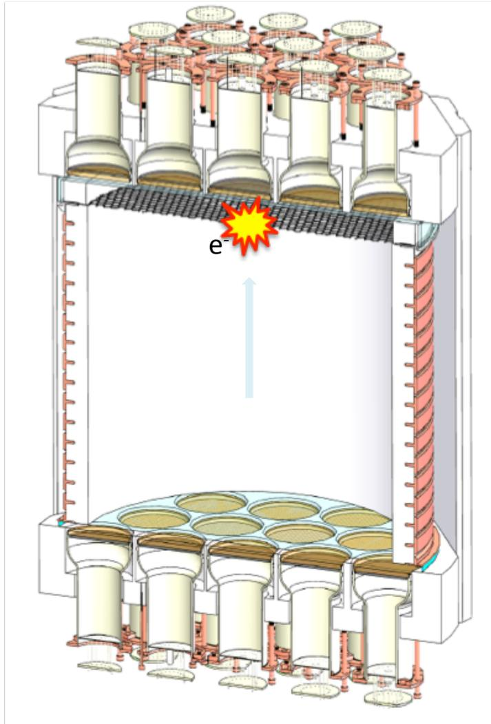
The electrons are extracted into the gas region, where they induce **electroluminescence (S2)**
