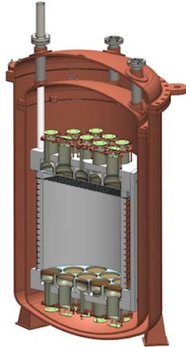
The DLAr-TPC technique is also foreseen for future large-scale **neutrino** detectors: (different energy range, different charge readout system, etc...)
