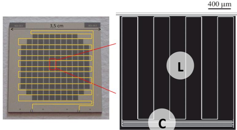
Kinetic Inductance Detectors (**KIDs**) are superconducting RLC resonators
