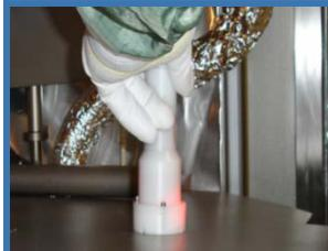
Particle Counter (airborne and from surfaces)
