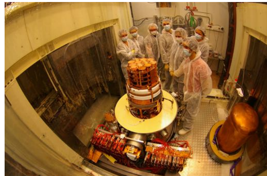
Installation of the 36 FID800 detectors at LSM
