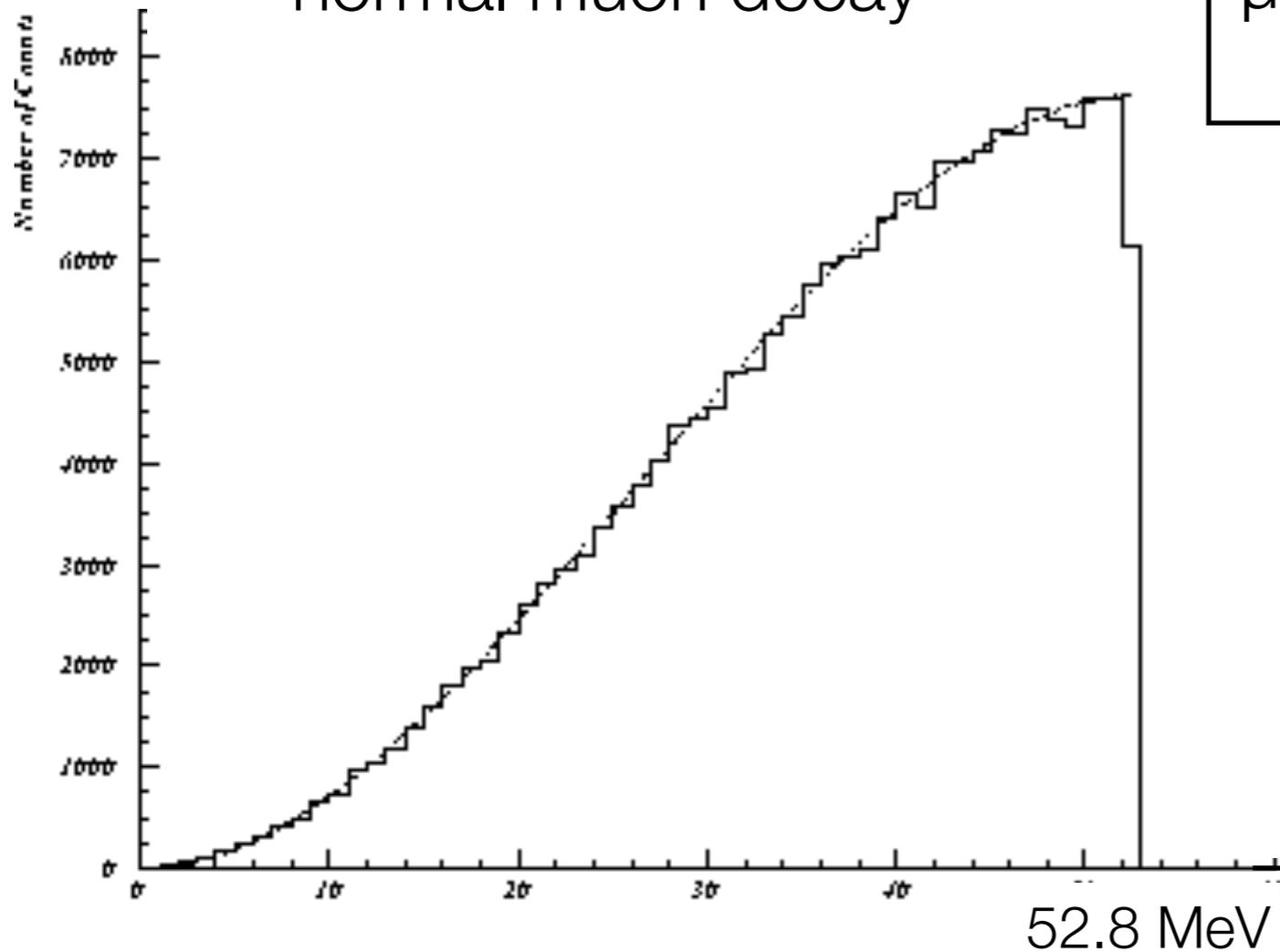
$\mu$ -e conversion and muon Michel decays are well separated.
