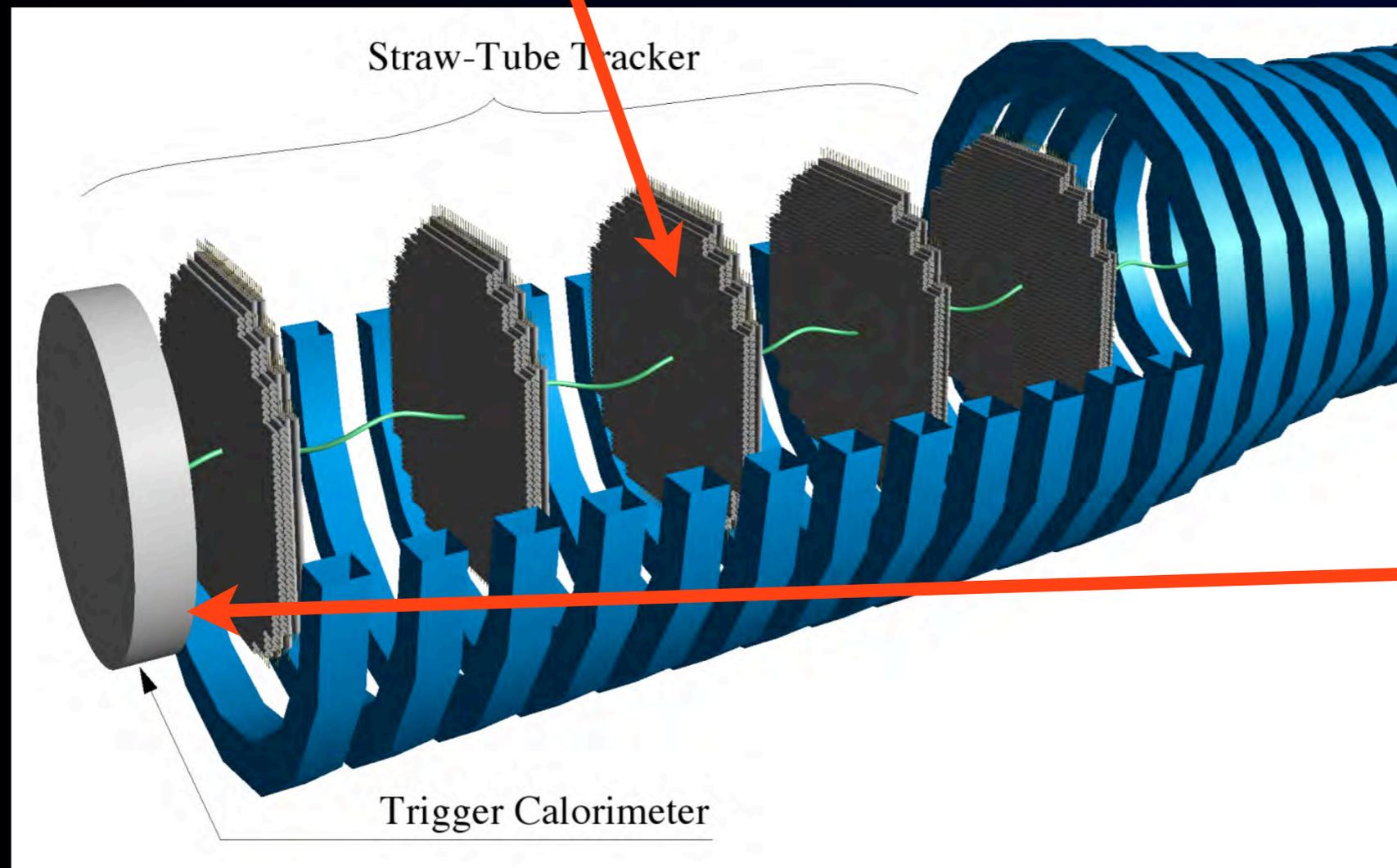
Electron calorimeter to measure electron energy, make triggers and give additional hit position.
