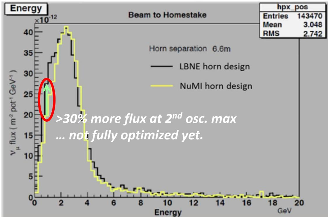
This is one example of significant improvements that are possible and needed, which new collaborators could bring into the design of the long-baseline neutrino facility beam design.
