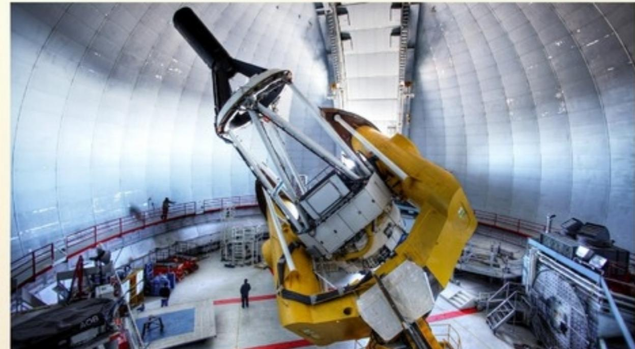
Equatorial mount with a prime focus cage
