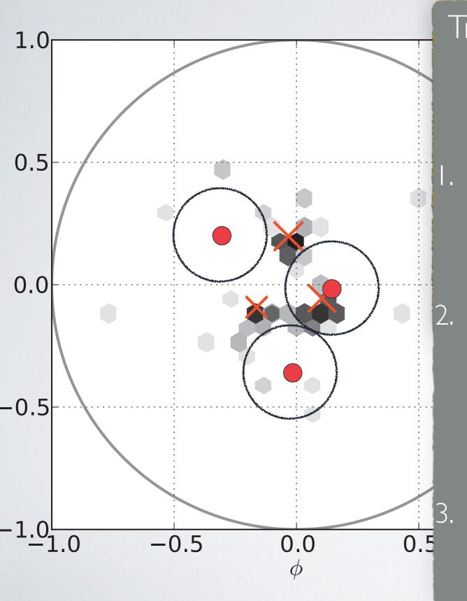
Try to match jet energy dist. to a parton structure of top decay products (TemplateTagger).
