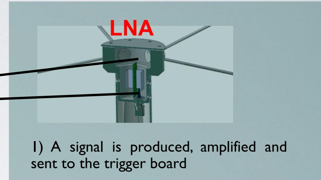
1) A signal is produced, amplified and sent to the trigger board
