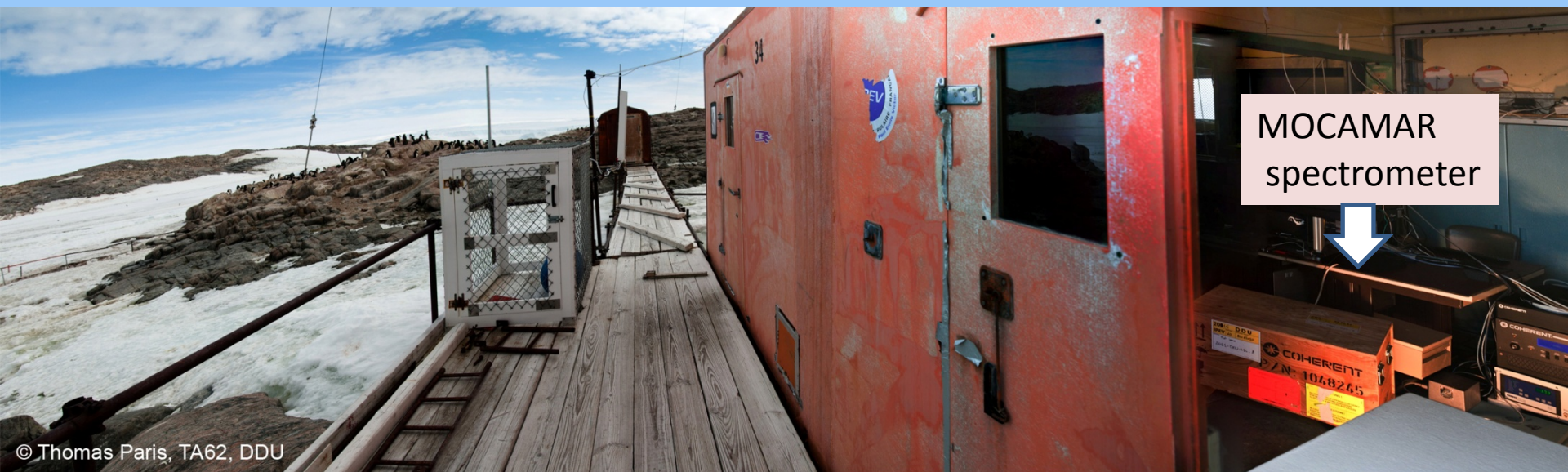
IO and NO 2 detection with a femtosecond-laser near-UV spectrometer installed at Dumont d'Urville (Antarctica) (collaboration LGGE) .
