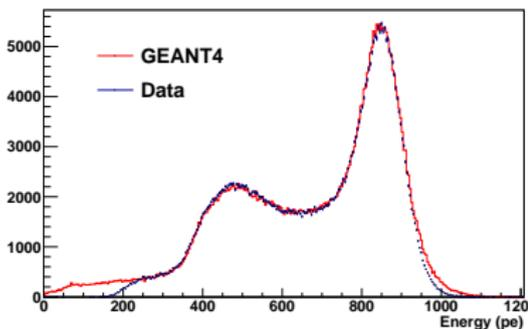
Neutron captures in target and shieldings
