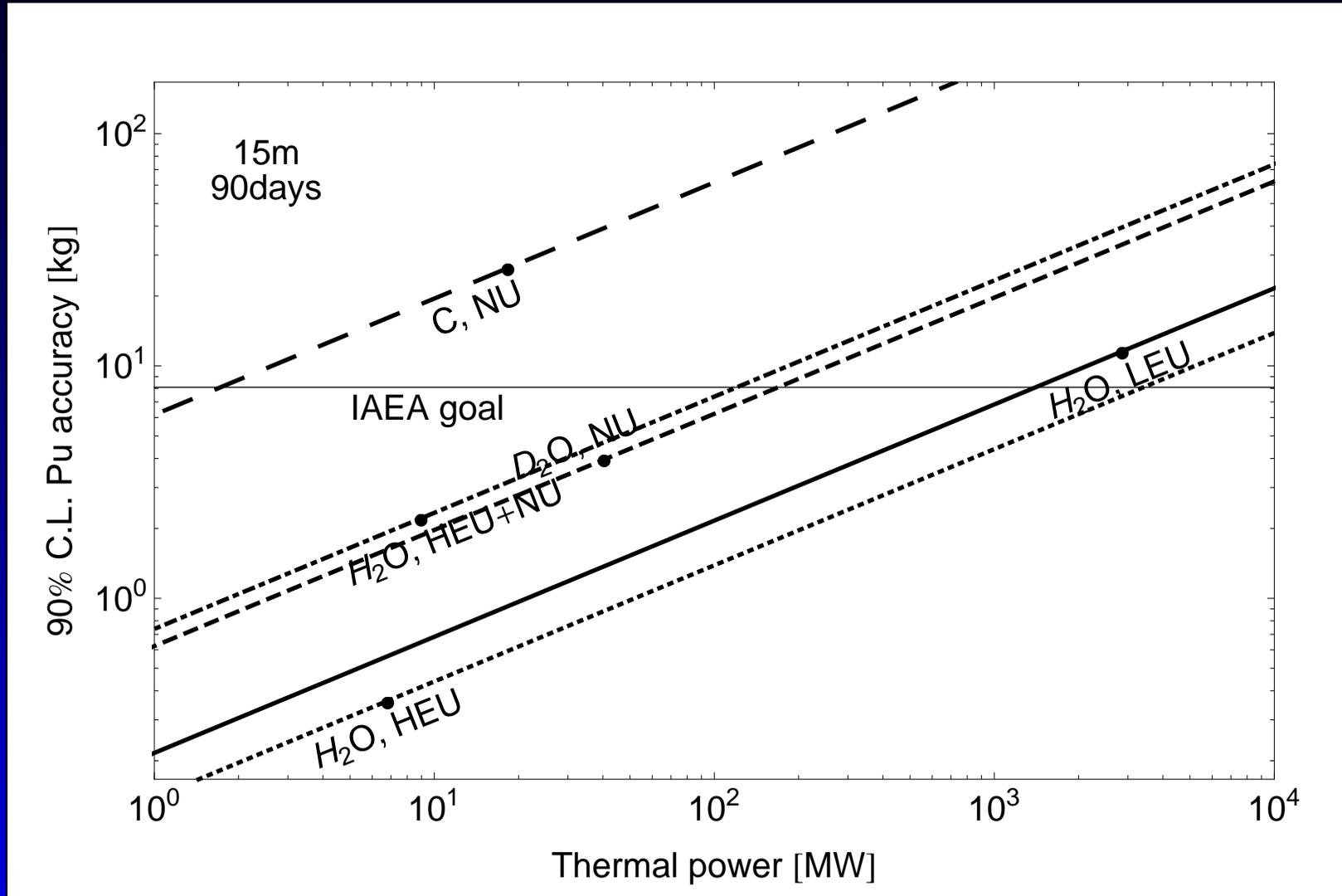
Fission fractions free in the fit. This is NOT based on a power measurement!
