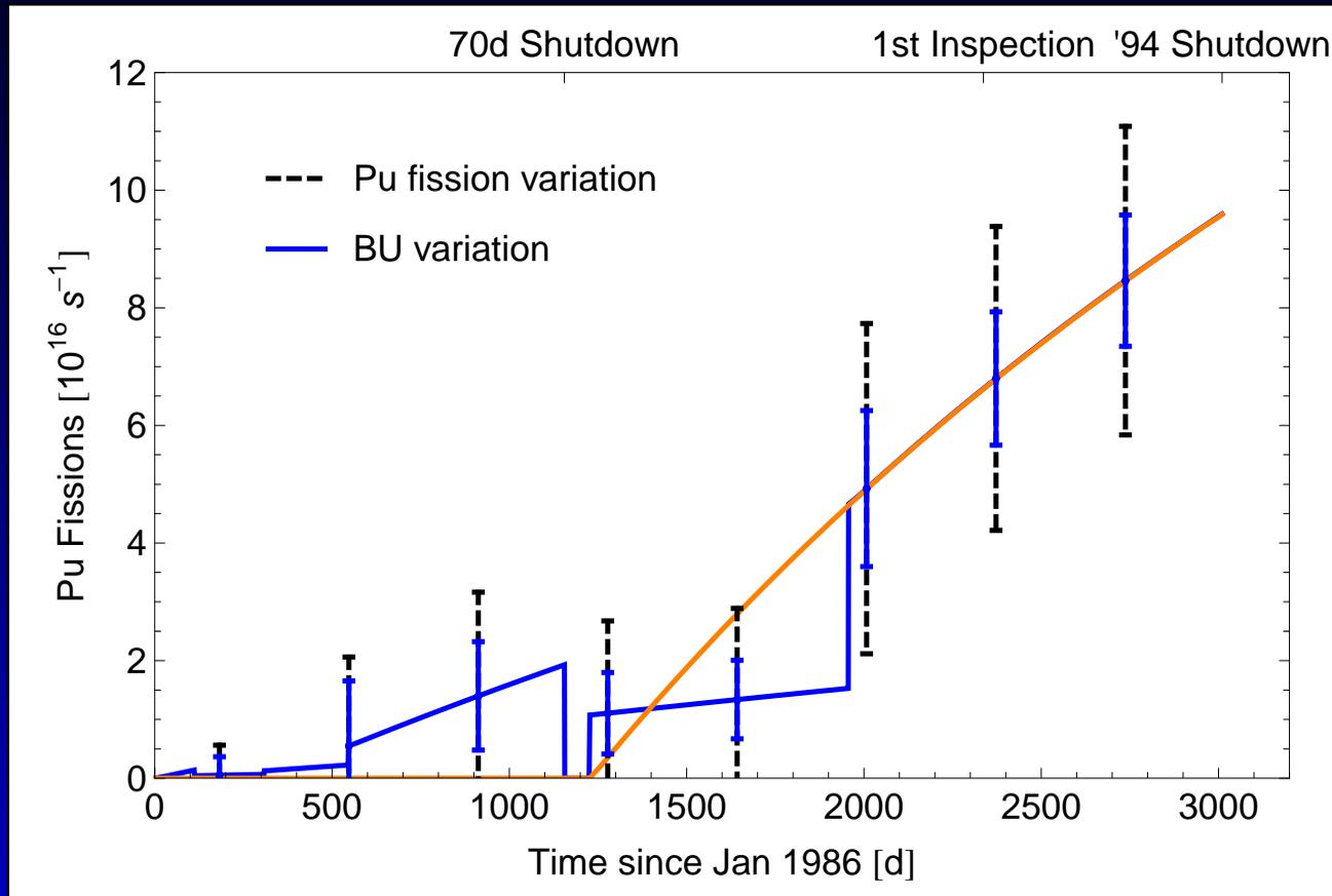
This demonstrates the gain in accuracy from using reactor physics to constrain the variation of FF.
