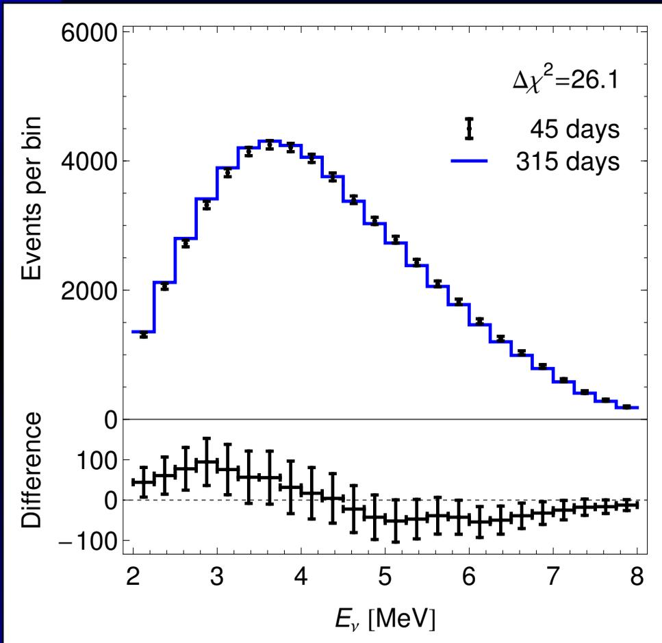
Comparing a reactor core at 45 days in the cycle to the same core at 315 days in the cycle
