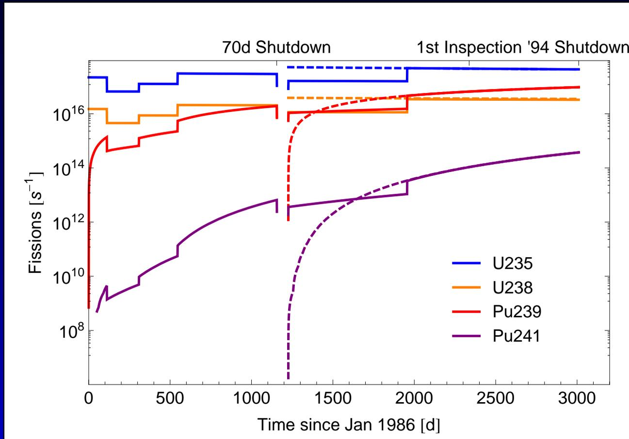
Full SCALE calculation in 0-d using a detailed power history to predict fission rates. Results of 2-d and 3-d simulations tend to be very similar.
