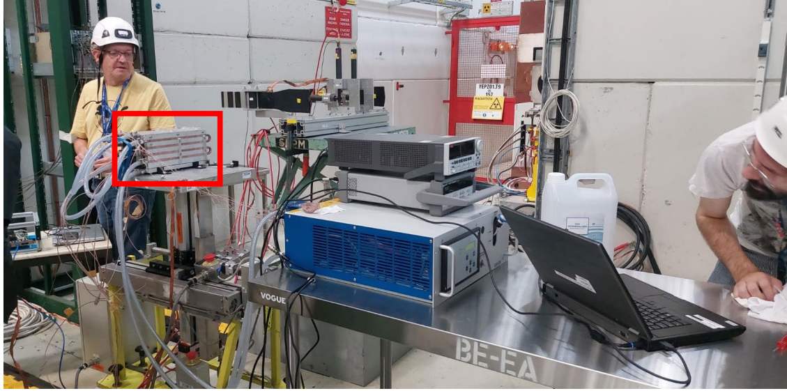
Figure 41: Setup of the beam test @CERN. The 5 \times 5 prototype is represented by the red rectangle in the setup. The chiller is placed on the table, with the AGILENT 34972A device positioned on top of it.
