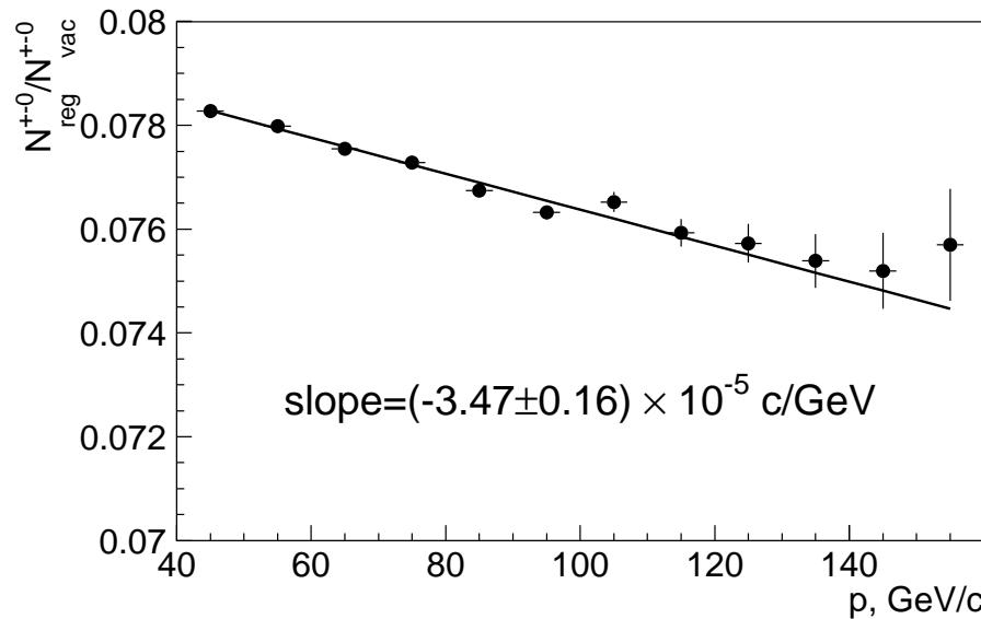
← Raw regenerator beam transmission as a function of kaon momentum.
