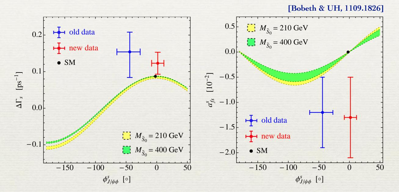
Even a light LQ fails to describe data & parameter space shrinks further for heavier LQs. Visible cosine-, sine-like correlations &  $\Delta\Gamma < (\Delta\Gamma)_{SM}$  model-independent feature
