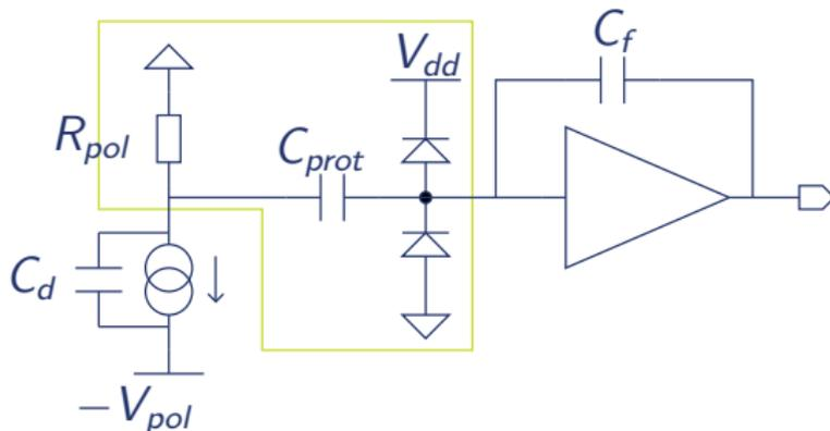
$C_{prot} > C_d \Rightarrow C_{prot} = 470 \text{ pF}$ .  $R_{pol} = 1..100 \text{ M}\Omega$
