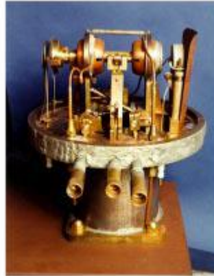
Fig. 7 The Varian Two-Cavity Klystron
