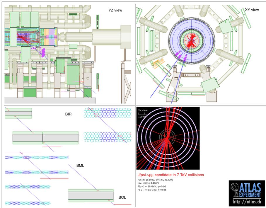
Figure 98: The same  $J/\Psi \rightarrow \mu\mu$ : in 2D projections and details of track reconstruction.
