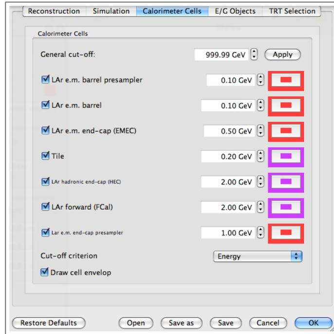
Figure 85: Selection of thresholds and cell envelopes to obtain the display of figure 86
