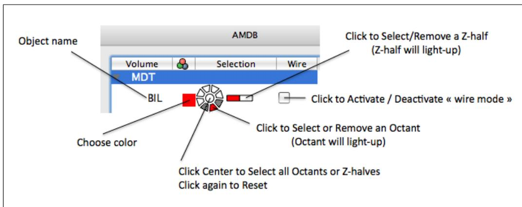
Figure 16: Illustration of the working of the Octant and Z-half selectors
