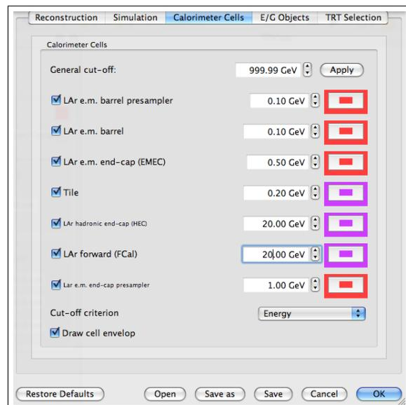
Figure 88: Selection of high thresholds in the *Set track parameters* window: energy thresholds of LAR HEC and FCal have been set to 20 GeV.
