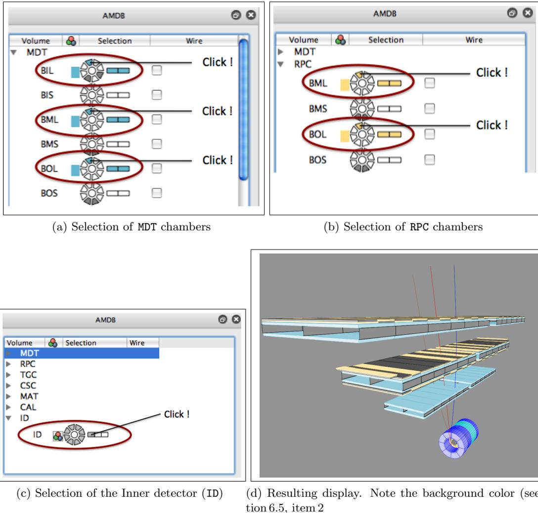
Figure 17: Illustration of the operations (a,b,c) resulting in the display shown in (d). The selections are highlighted inside a red ellipse.
