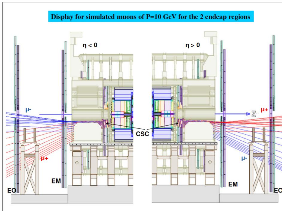
Figure 92: Illustration of the charge asymmetry of forward low energy muons in 900 GeV collision data. The intricate acceptance effect is illustrated with generated positive (red) and negative (blue) muons in the forward regions.
