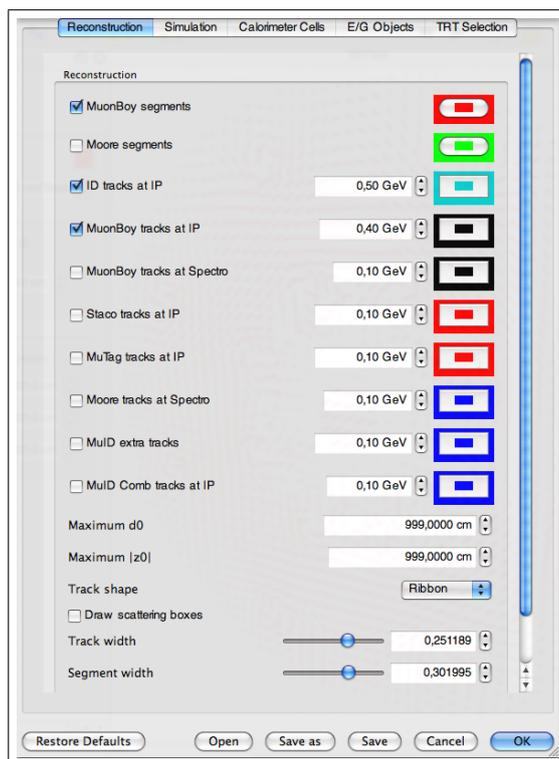
Figure 6: *Set track parameters* window. The parameters shown here - for the *Reconstruction* tab - are those of the predefined parameters of file `Zmumu4023.p2ts` mentioned below. See Appendix E.5.1 for the content of all 5 tabs.
